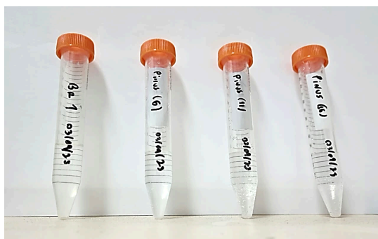
Figure 1. Photo of the solutions after sample decomposition through microwave assisted using 100 mg pine needle replicates and 3 mL of 30% (m/m) H 2 O 2 .
